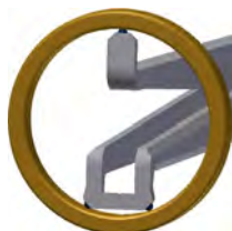
Tasterform / probe contacts 2 Kugel / Ball Ø 1,0mm
